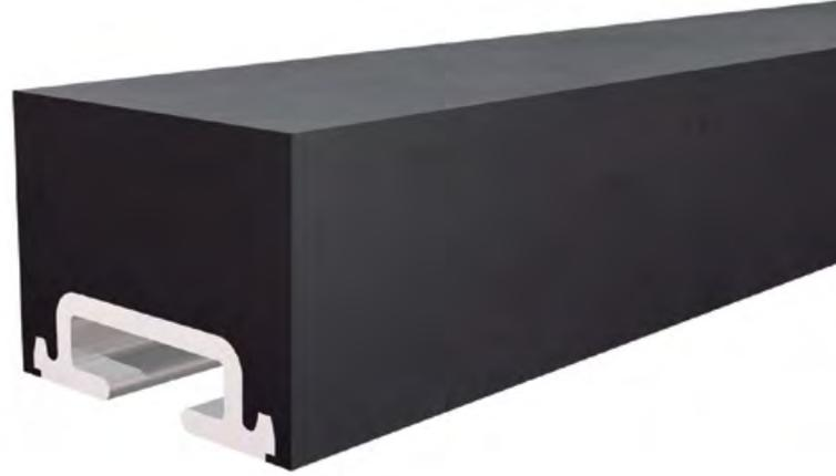
Excellent wear resistance in applications with both impact and sliding wear. The embedded aluminum profile allow for fewer fixing points than steel-reinforced wear plates. Trellex WB wear bars reduce noise and vibrations, and are lighter compared to conventional steel shrouding.
