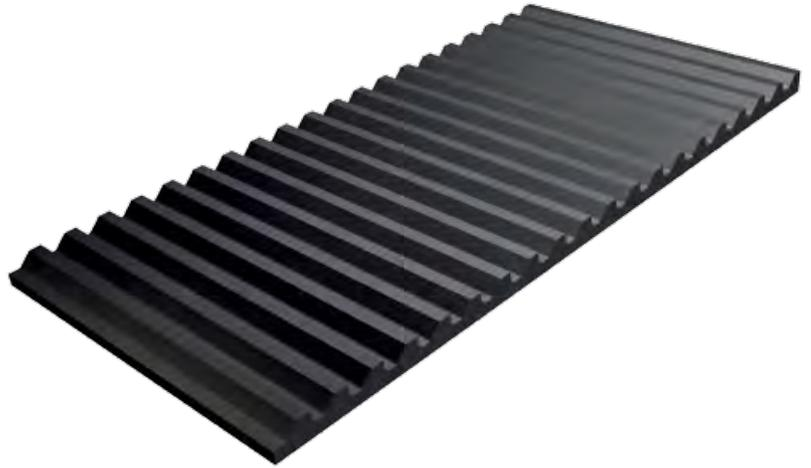
Excellent wear resistance in applications with both impact and sliding wear. The steel backing guarantees secure fixing so that the wear plates remain together even if the lining is exposed to extremely abrasive and sharp particles. The serrated surface has been designed to provide optimal life for material with impact angles between 15° and 50°. Trellex SP wear plates reduce noise and vibrations, and are lighter compared to conventional steel lining.
