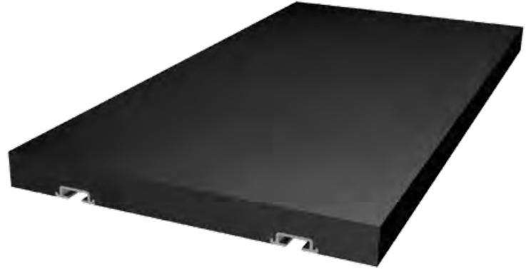
Excellent wear resistance in applications with both impact and sliding wear. The vulcanized aluminum profiles allow for fewer fixing points than steel-reinforced wear plates. Trellex PT wear plates reduce noise and vibrations, and are lighter compared to conventional steel lining.
