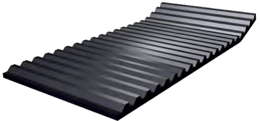
Trellex Flexback shows excellent wear resistance in lighter and medium applications. The reinforcement makes it possible to construct self-supporting channels and chutes with simple supports of angle iron and flat iron. The Flexback products reduce noise and vibrations, and are lighter compared to conventional steel lining. Trellex Flexback is available in rubber and polyurethane.
