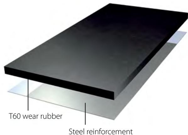
Excellent wear resistance in applications with both impact and sliding wear. The steel backing prevents small particles getting in under the lining and guarantees secure fixing. Wear plates reduce noise and vibrations, and are lighter compared to conventional steel lining.
