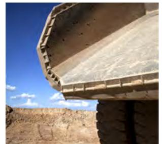
**Sheeting** Trellex wear sheeting has proved a long wear life in comparison with other wear materials like steel. Fewer stops and less production losses increase your profitability. Depending on application you can choose from rubber or polyurethane wear sheeting.
