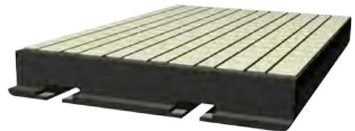
Trellex Poly-Cer is designed to be extremely resistant to abrasion even in high material flows and speeds. The unique design of ceramic inserts improves wear life and impact resistance. Trellex Poly-Cer is made of T60 wear rubber with built-in ceramics and enhanced with fixed hot-vulcanized steel reinforcement.
