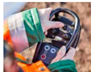
Remote controller for crawler tracks as standard and optional extra controller for other functionalities
