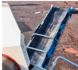
Wide fines conveyor and possibility for two-way split (optional)
