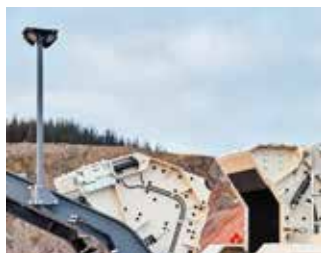
Working lights as standard for better work ergonomics and safety
