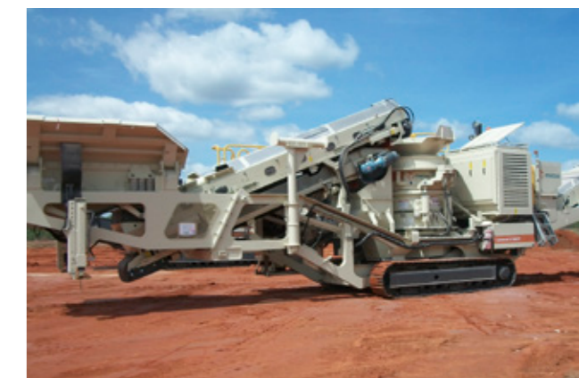
Lokotrack LT300HP is available with either a belt feeder or alternatively with a vibrating grizzly feeder.
