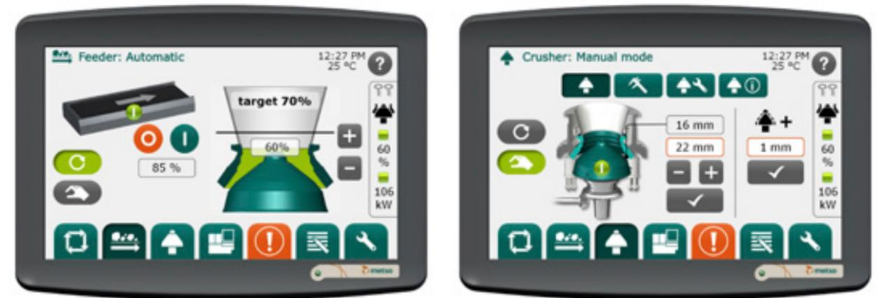
Metso IC crusher automation adjusts the crushing process automatically. You can also benefit from the special fine-adjustment features that enable easy crushing process optimization.
